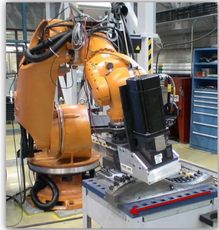
Process forces: F_x = 1,2 \text{ kN} , F_y = 1,1 \text{ kN} , F_z = 10 \text{ kN} Hybrid position/force control
