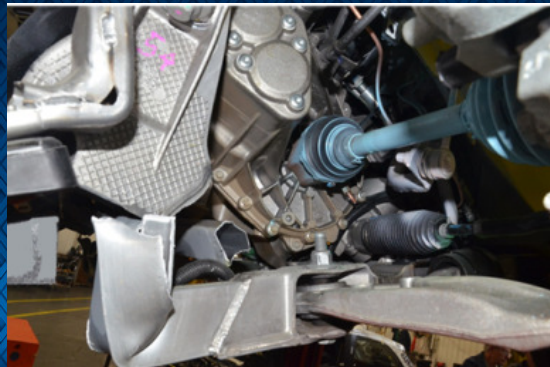
Subframe – Extrude Aluminum Portion
