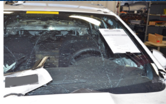
Laminated Chemically Toughened Windshield
