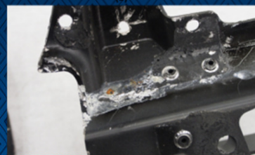
Mg castings, same surface, different sealer
