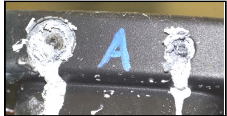
Corrosion Results of Attaching Screws after 240 Hr. ASTM B117 Salt Spray Exposure
