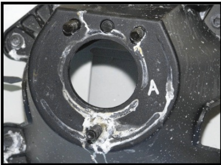
Prototype with no mylar isolator after 240 Hr ASTM B117 Salt Spray exposure
