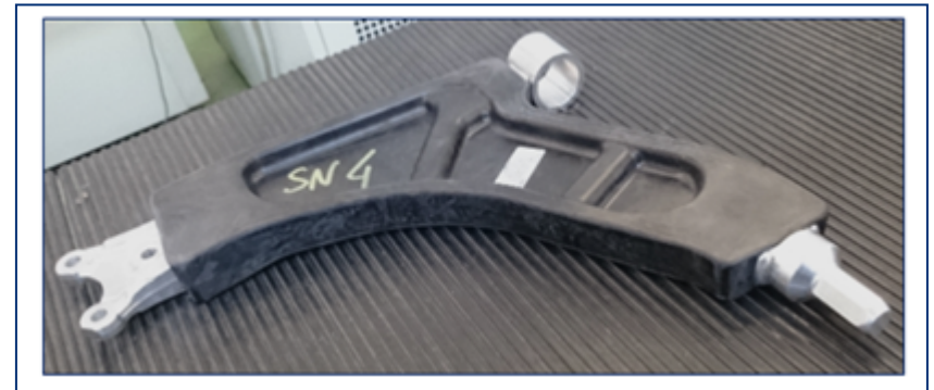
MMSS Composite Suspension Arm
