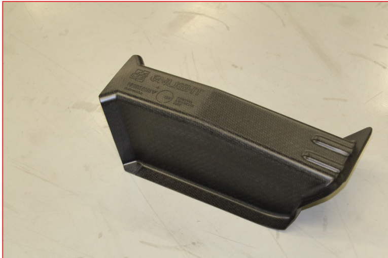
Thermoformed GF-PA6 sheet, weight 1,16 kg
